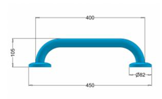
Product guarantee for practical competence, access to the area and the washbasin, shower toilet. Straight handrails can be a tool not only in bathrooms but also wherever there is one - as long as the assembly area has been appropriately needed. The 444 handrail is made of AISI304 steel and is available in two surface variants (satin or polished finish).
