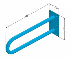
Arch fixed wall for disabled people, length 800 mm. generalpurpose, made of polished stainless steel tube or matt 32 mm diameter. We use this type of handrail in the washbasin, shower and toilet area.
