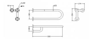
Left basin handrail for disabled people, 550 mm long, generalpurpose, made of stainless steel tube, 25 mm diameter. We use this type of handrail in the washbasin. The handles are equipped with masking rosettes with a click system, which allows mounting the masking rosette without the use of mounting glue.
