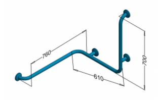
Left-hand shower handrail for people with disabilities 760x610x700mm long, general-purpose, made of polished or matt stainless steel 32 mm diameter. We use this type of handrail in the shower area. The handles are equipped with masking rosettes with a click system, which allows mounting the masking rosette without the use of mounting glue.
