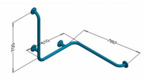
Right-hand shower handrail for people with disabilities 700x610x760mm long, general-purpose, made of polished or matt stainless steel 32 mm diameter. We use this type of handrail in the shower area. The handles are equipped with masking rosettes with a click system, which allows mounting the masking rosette without the use of mounting glue.
