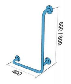
Handrail for the disabled angled left, mounted to the wall, 600x400 mm long, made of 25 mm diameter carbon steel tube, powdercoated, white. We use this type of handrail in the shower and toilet area. The distance of the handrail from the wall to the center of the tube is 90 mm.
