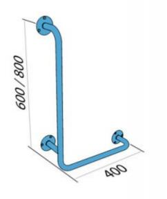
Handrail for the disabled angled right, mounted to the wall, 600x400 mm long, made of 25 mm diameter carbon steel tube, powder-coated, white. We use this type of handrail in the shower and toilet area. The distance of the handrail from the wall to the center of the tube is 90 mm.
