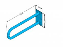
Handrail for disabled people, arched, fixed, 600 mm long, generalpurpose, made of 32 mm diameter carbon steel tube, black powder coated. We use this type of handrail in the washbasin, shower, and toilet area.
