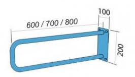
Handrail for disabled people, arched, fixed, 600 mm long, generalpurpose, made of 25 mm diameter carbon steel tube, white powder coated. We use this type of handrail in the washbasin, shower, and toilet area.
