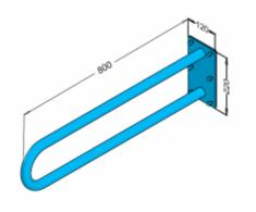
Handrail for disabled people, arched, fixed, 800 mm long, generalpurpose, made of 32 mm diameter carbon steel tube, white powder coated. We use this type of handrail in the washbasin, shower, and toilet area.
