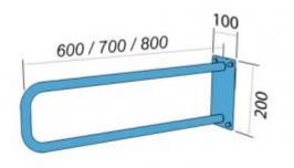
Handrail for disabled people, arched, fixed, 800 mm long, generalpurpose, made of 25 mm diameter carbon steel tube, white powder coated. We use this type of handrail in the washbasin, shower, and toilet area.
