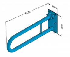
Handrail for disabled people, arched, tilting, wall-mounted, length 600 mm, general-purpose, made of 32 mm diameter carbon steel tube, white powder coated. We use this type of handrail in the washbasin, shower, and toilet area.
