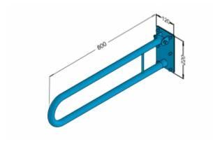
Handrail for disabled people, arched, tilting, wall-mounted, length 800 mm, general-purpose, made of 32 mm diameter carbon steel tube, white powder coated. We use this type of handrail in the washbasin, shower, and toilet area.
