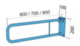
Handrail for disabled people, arched, tilting, wall length 800 mm, general-purpose, made of 25 mm diameter carbon steel tube, black powder coated. We use this type of handrail in the washbasin, shower, and toilet area.
