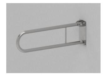
**Arched and tilted handrail for the diabled**, makes everyday actions easier and rises safety for eldery and disabled people. While using sanitary products like shower, washbasin or toilet. Straight handrail for disabled is made of ø25 mm tube (thicness 1,5 mm), made of stainless steel AISI 304. It hac PZH and CE certificate and entry in the register of medical devices. Max. weight is 180 kg. For general use
