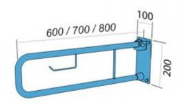
Handrail for people with disabilities arched, tilting, a wall with space for paper, 700 mm long, general-purpose, made of 25 mm diameter carbon steel tube, powder-coated, white. We use this type of handrail in the wc area.
