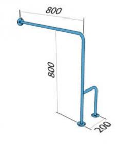
Left handrail for disabled people, wall left, 800x800 mm long, made of 25 mm diameter carbon steel tube, white powder coated. We use this type of handrail in the shower and toilet area.
