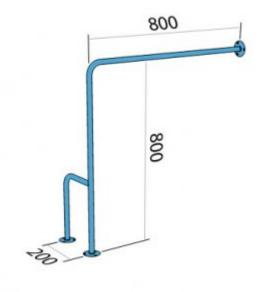
Right handrail for disabled people, wall left, 800x800 mm long, made of 25 mm diameter carbon steel tube, white powder coated. We use this type of handrail in the shower and toilet area.
