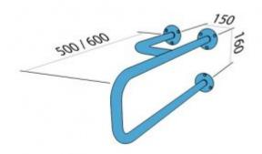
Left handrail for washbasins (tripod) left, mounted to the wall, 500 mm long, made of 25 mm diameter carbon steel tube, powdercoated, white. We use this type of handrail in the washbasin.
