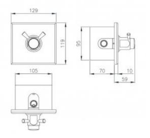
Mounting box made of stainless steel. Designed for mounting 9005MIX PLUS valve
