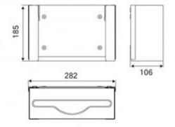
Recess paper towel dispenser made of matt stainless steel. Designed for built-in behind a mirror or wall. The capacity of the tray is about 300-400 ZZ folded towels.
