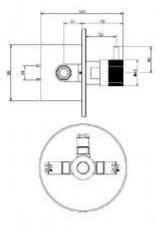
Timed, self-closing mixer used for water supply. The mixer is built into an elegant mounting box, which, apart from the visual value, has a protective nature - AISI 304 stainless steel finish and vandalproof protection. The 9095MIXC mixer is adapted to double 1/2 "connection with the possibility of reduction via a 3/8 &HASH39;half unions. The connection is two-phase, which means that cold and hot water should be connected to the mixer. Moreover, the mixer has a 15-year warranty.
