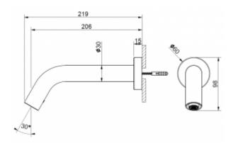
The touchless washbasin faucet 2519B is designed for wall mounting, including installation on plasterboard surfaces. Its construction allows for quick and hassle-free installation, while the built-in infrared sensor automatically activates the water flow when motion is detected within its range.
