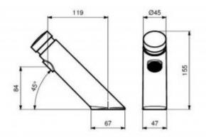
The self-closing basin tap with a moving aerator. The body is made of chrome-plated brass. The tap has one G1 / 2 connection. A single outflow of water takes about 15 seconds (at a water pressure of 3 bar). The amount of water used is 6 l / m. The minimum connection pressure is 1 bar, the maximum is 6 bar. It is worth adding that the recommended connection pressure should be 2-4 bar.
