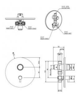
Timed, self-closing mixer used for water supply. The 9095MIXC mixer is adapted to double 1/2 "connection with the possibility of reduction via a 3/8 &HASH39; half unions. The connection is twophase, which means that cold and hot water should be connected to the mixer.
