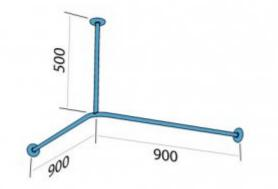
The shower curtain rod is made of carbon steel tube with a diameter of 25 mm, powder-coated, white enameled, 900 x 900 x 500 mm. This type of shower bar is designed for a shower area and in combination with the PD90 non-threshold shower tray is the optimal solution for people with disabilities.
