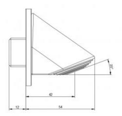
Solid spray spout. Made of chrome-plated brass. The spout makes it resistant to vandalism. The slim design definitely makes it difficult for the user to devastate the screed by hanging on it, which can result in the screed being pulled out of the wall. The strainer made of plastic with the option of reducing water pressure. Equipped with a masking rosette.
