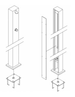
Column shower set made of AISI 316 stainless steel, adapted for floor mounting. The shower set 9220 has one 1/2 &HASH39; connection for cold or mixed water, with a standard water flow time of about 30-50 seconds ± 1 second. The flow system is enriched with a safety device that automatically shuts off the water flow after 15 seconds at a pressure of 3 bar.
