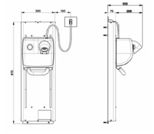
Slider for adjusting the height of pool dryers. The slider has been adapted to the Magnum H series dryers. for moisture, e.g. swimming pool changing rooms. The offered slider has a total size of 320 x 76 x 975 mm (without the dryer installed).
