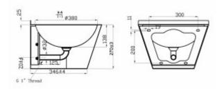
Quadrangular washbasin made of stainless steel, designed for wall-mounting. Has a special edge, which protects the wall from water and mounting hole for battery assembly.
