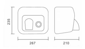
Professional hand and hair dryer, activated at the touch of a button. Intended for swimming pools, hospitals, medical, treatment and dental offices. The casing of the offered dryer is made of stainless steel, which is highly resistant to vandalism. In addition, the steel housing is waterproof and has an IPX1
