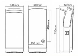
It is the first crevice dryer in the world in a stainless steel housing. The vertical hand dryer in white color finish is equipped with a HEPA filter system, has a larger hand drying gap, which is made in antibacterial technology, has a built-in water tank eliminating the accumulation of dripping water.
