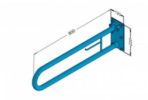
Handrail for disabled people, arched, tilted, wall with space for toilet paper, 800 mm long, general purpose, made of 32 mm diameter carbon steel tube, powder coated, white. We use this type of handrail in the wc area.
