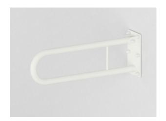
Handrail for disabled people, arched, tilting, wall-mounted, length 700 mm, general-purpose, made of 32 mm diameter carbon steel tube, white powder coated. We use this type of handrail in the washbasin, shower, and toilet area.
