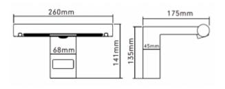
A countertop dryer with a built-in photocell battery is a product that is most often used in large public bathrooms. The offered set is made of brass. In addition, the steel housing is waterproof and has IP24 protection.
