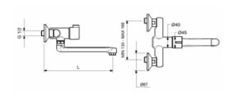
Wall-mounted tap with built-in thermostatic mixer TMV3 with limited water temperature to 41°C. The faucet body is made of corrosion-resistant chrome-plated brass. In the central part of the body there is a button that activates the water flow, a water temperature regulator and a swivel spout. Spout has a built-in
