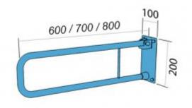
Handrail for disabled people, arched, tilting, wall-length 700 mm, general-purpose, made of 25 mm diameter carbon steel tube, white powder coated. We use this type of handrail in the washbasin, shower, and toilet area.
