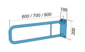
Handrail for disabled people, arched, tilting, wall-length 700 mm, general-purpose, made of 25 mm diameter carbon steel tube, black powder coated. We use this type of handrail in the washbasin, shower, and toilet areas.
