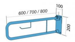
Handrail for people with disabilities arched, tilting, a wall with space for paper, 600 mm long, general-purpose, made of 25 mm diameter carbon steel tube, powder-coated, white. We use this type of handrail in the wc area.
