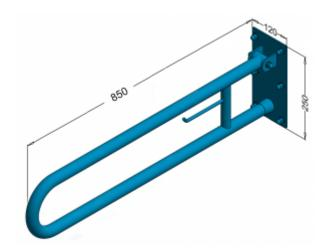
Tilting arch handrail with a place for toilet paper for disabled people, length 850 mm, general-purpose, made of polished stainless steel tube or matte 32 mm diameter. We use this type of handrail in the wc area.
