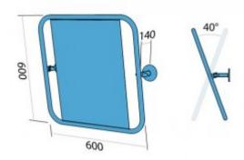
Tilting mirror for the disabled in a full-frame, made of 25 mm diameter carbon steel tube, powder-coated, white. We use this type of mirror in the washbasin.
