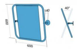
Tilting mirror in full frame for people with disabilities, 600x600 long, general purpose, made of polished or matt stainless steel fi 25 tube diameter. We use this type of mirror in the wash basin. Equipped with masking rosettes with a snap-in system, which allows the masking rosette to be mounted without the use of mounting glue.
