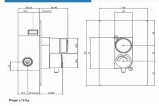
Shower timer with thermostatic mixer. Temperature regulation by means of a knob located below the start button. Possibility of safe water temperature regulation thanks to anti-scalding protection preventing exceeding the permissible temperature of 38°C. A single water flow can last 15-25 seconds (water pressure 3 bar), with water consumption of approx. 6 l / m. The water connection pressure can be 0.5 - 6 bar, however, the recommended connection pressure should be 2-4 bar.
