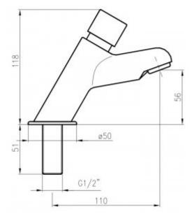
A push-button timer with a one 1/2 &HASH39; connection for cold or mixed water is a product that will be perfect for medium-sized public spaces such as gyms, saunas, swimming pools, hostels, and others. The faucet should be connected to the cold or warm premixed water system.
