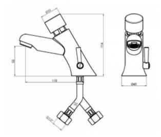
A self-closing basin mixer with a push button is made of chromeplated brass is an ideal solution for public spaces such as swimming pools, saunas, shopping centers, hotels, and others. The 9007 tap is equipped with a mixer and two 1/2 "connections. Starting the water flow is possible thanks to the button, the water flow time is from 8-12 seconds  $\pm$  5 seconds (depending on the settings).
