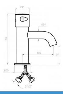
Washbasin timer with manual mixer adjustable in the button. This type of solution makes temperature regulation intuitive and simple. Thanks to its innovative appearance, it works perfectly in bathrooms of high standard rooms such as restaurants, banquet rooms and hotels
