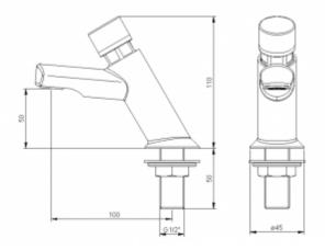
A self-closing basin with a push button is made of chrome-plated brass is an ideal solution for public spaces. The 8250 tap is equipped with one 1/2 "connection. Starting the water flow is possible thanks to the button, the water flow time is from 8-12 seconds  $\pm$  5 seconds (depending on the settings).
