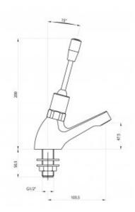
The 9001L basin tap with lever is a classic product for mixed water. The body is made of solid brass covered with chrome. The whole has one G1 / 2 connection and elements regulating the water flow. The mentioned elements are:
