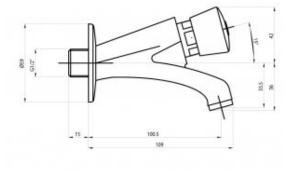
Wall-mounted washbasin timer with one G1 / 2 connection for cold or premixed water. The body of the faucet is made of solid brass covered with a layer of chrome. The built-in spout is equipped with a standard strainer to regulate the water stream.
