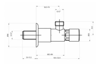
Shower self-closing tap with one water connection G1/2 for cold or mixed water. The single flow of water is 15-25 seconds with a water pressure of 3 bar. The amount of water that is used for a single outflow is about 6 l / m. In addition, the water connection pressure can be 0.5 - 6 bar, the recommended connection pressure should be 2-4 bar.
